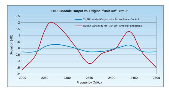
*Figure 4* shows the THPR's output across frequency, which is accurate to approx 0.3 dB. The drift of all the components in the system is managed by the THPR's active power control and yields a very predictable, robust, and long-range link. In short, achieving the power setting necessary to meet a desired link margin is best achieved with a turnkey ISR link solution, as all previously uncontrollable radio/ amplifier variability is compensated for internally.
