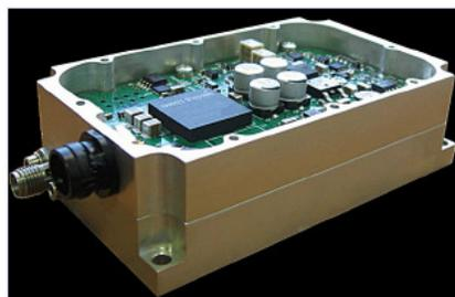
**Figure 2: The DC supply board allows a wide input voltage range.**
