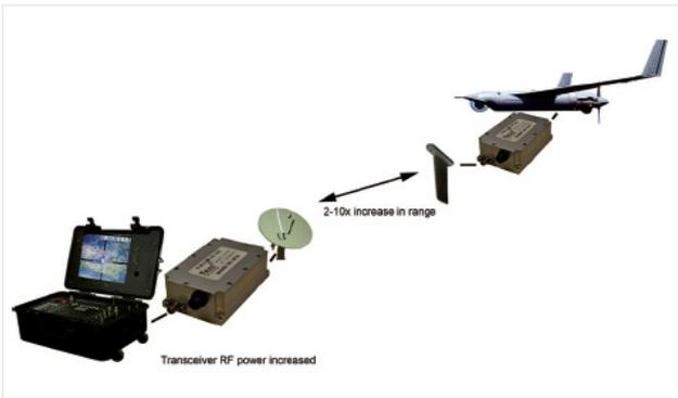
Figure 3: A typical scenario in which the TTRM1010 is employed to extend the range of an Unmanned Aerial Vehicle, (UAV) or Unmanned Ground Vehicle (UGV).
