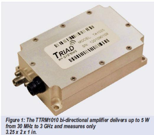
**Figure 1: The TTRM1010 bi-directional amplifier delivers up to 5 W from 30 MHz to 3 GHz and measures only 3.25 x 2 x 1 in.**
