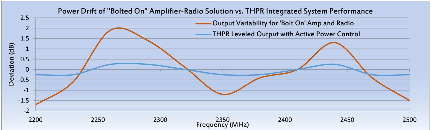
The THPR Series of range-enhanced radios employ **Active Power Control** to ensure that the both the **RF Output Power and SNR** delivered to the antennas remains **ultra-stable** in the presence of fluctuations arising from the above factors. This results in:
